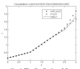
*Fig. 3.* The distribution of Ca concentration *c* depending of vertical coordinate *z* in three points: x = l/2, y = L/2; *i*=1, *j*=2; *i*=M (*x*=1), *j*=1
