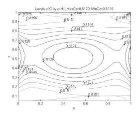
*Fig. 4.* The distribution of Fe concentration c in the (x; y) plane (Levels of c) by z = H1
